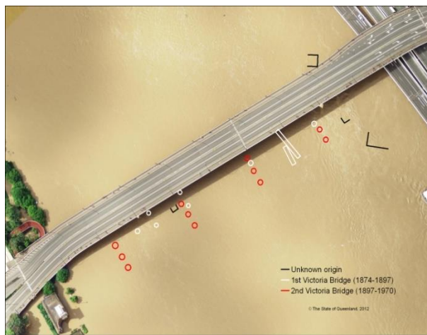
Figure 24 – Extant remnants of earlier Victoria Bridges
