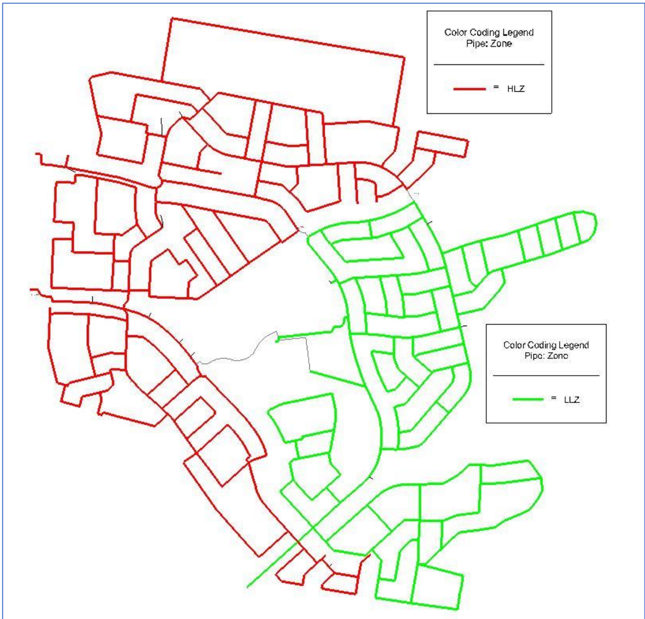
Figure 7.4: HLZ and LLZ Water Network
