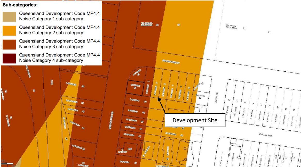
Plate 3: Default road traffic Noise Categories for the Development (Source: Brisbane City Council)
