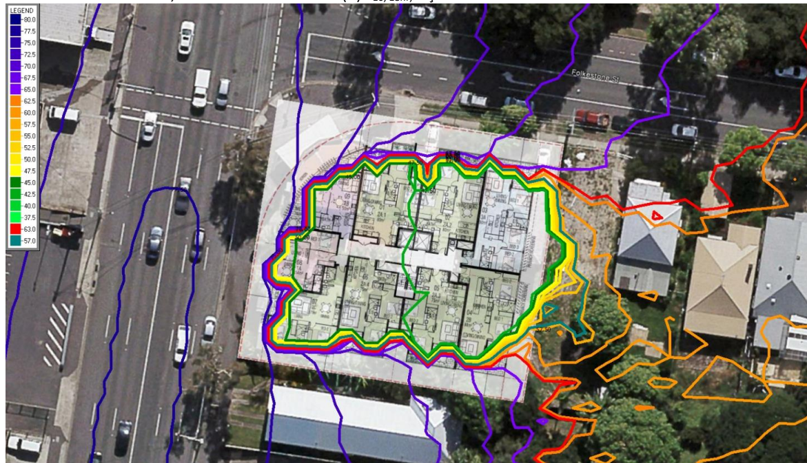
Plate B5: Noise contours, Level 5. Levels are in dB(A) L_{10, 18hr} , façade-affected.
