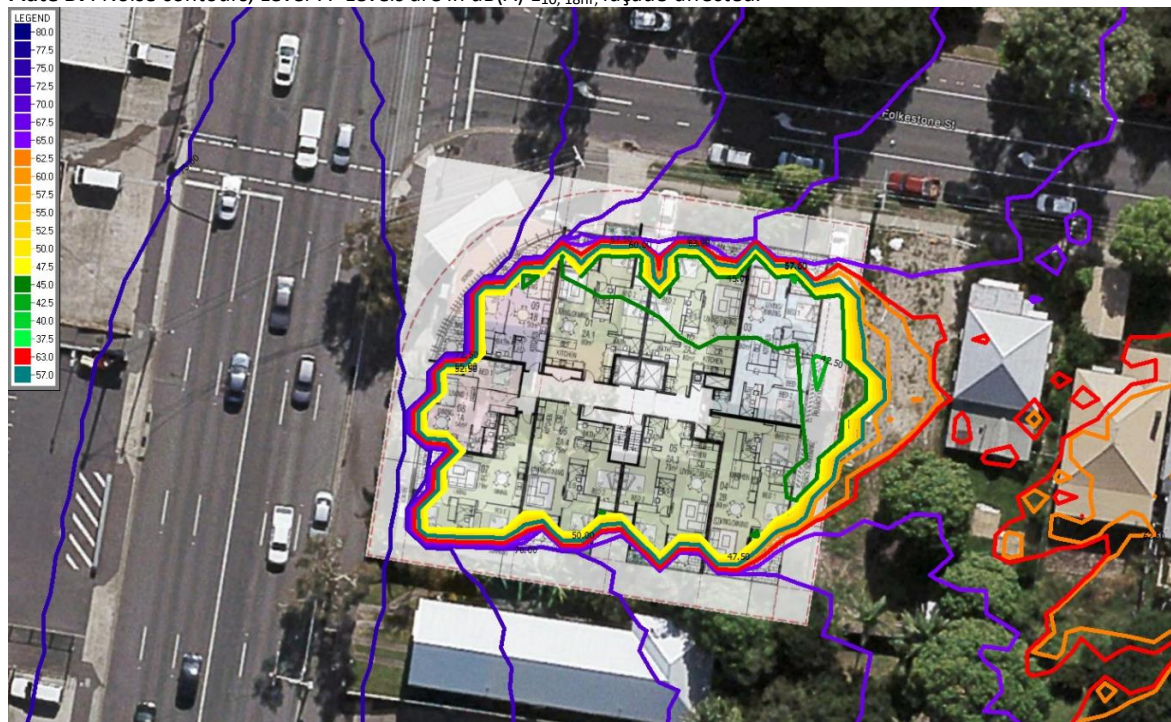
Plate B7: Noise contours, Level 7. Levels are in dB(A) L_{10, 18hr} , façade-affected.
