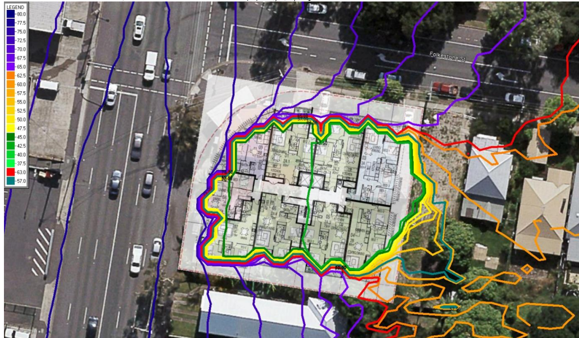
Plate B4: Noise contours, Level 4. Levels are in dB(A) L_{10, 18hr} , façade-affected.
