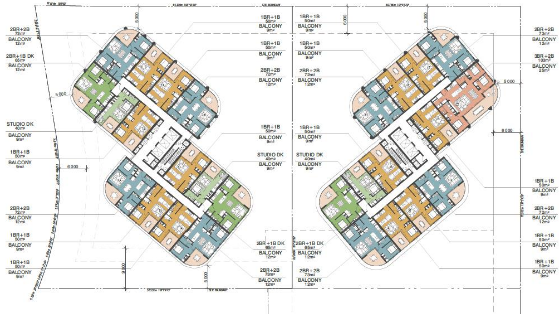
Figure 6: Typical Tower floor plan, showing balconies.
