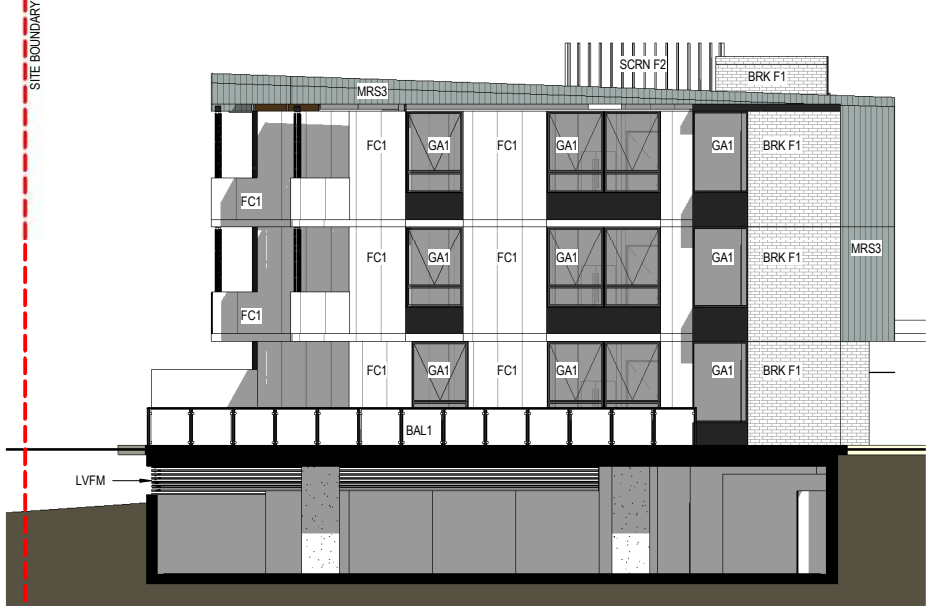
4 Building 02 - Elevation 4 DA 102 1: 100
