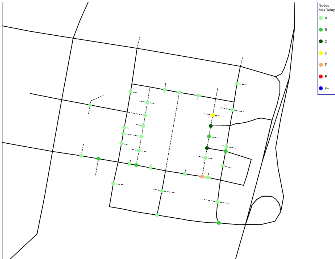
Figure 6-11: 2031 Nodes Level of Service PM Peak (Unsignalised)
