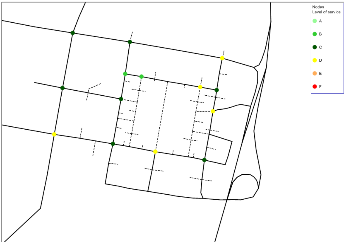
Figure 6-8: 2031 Intersection Level of Service AM Peak (Signalised)
