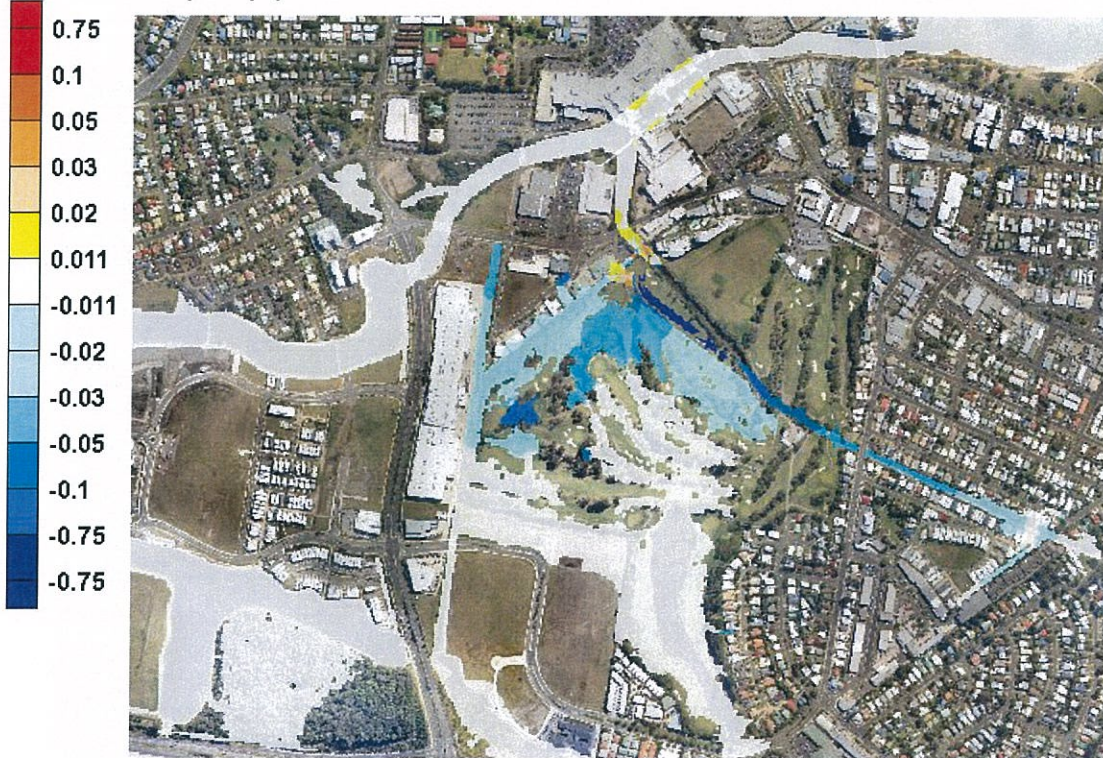
Figure 3 Stage 1 Temporary Works 10% AEP Flood Impact
