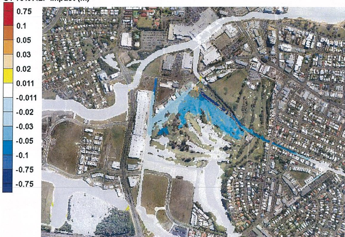
Figure 2 Stage 1 Temporary Works 18% AEP Flood Impact
