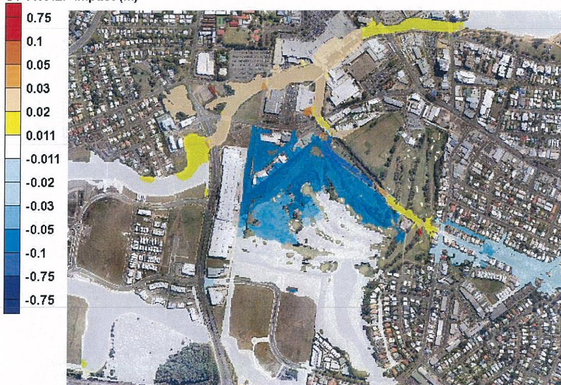
Figure 6 Stage 1 Temporary Works 1% AEP Flood Impact
