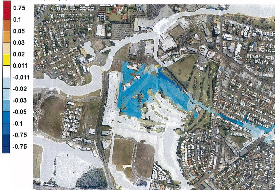
Figure 5 Stage 1 Temporary Works 2% AEP Flood Impact
