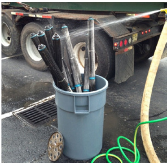
Rinsing the dirty cartridge tentacles with a low-pressure garden hose, and using a garbage bin to capture the run-off
