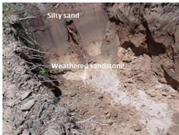
Photo: Silty sand over weathered sandstone
