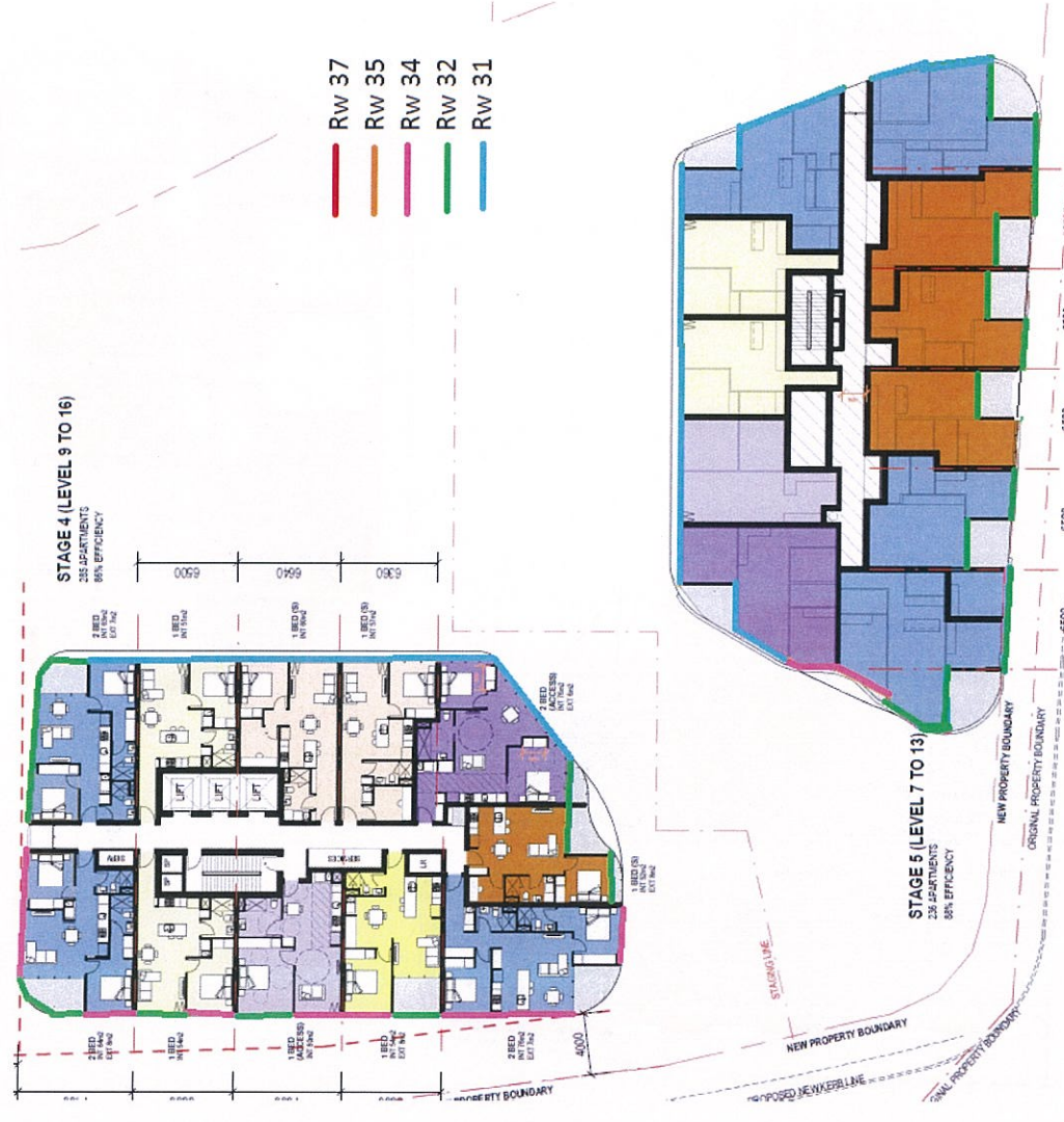
Figure 8: Glazing requirements Stage 4 Level 9 to 16, Stage 5 Levels 9 to 16
