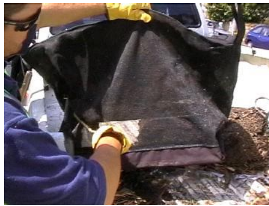
Plate 27 A clean used filter bag
