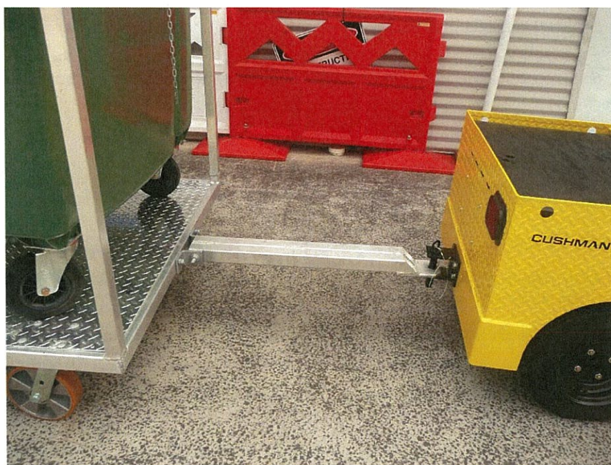
Figure 2: Attachment between 5k ride-on tug and aluminium trailer.
