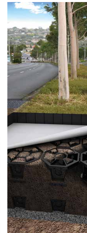
structural soils under pavements to promote full growth of the urban jungle
