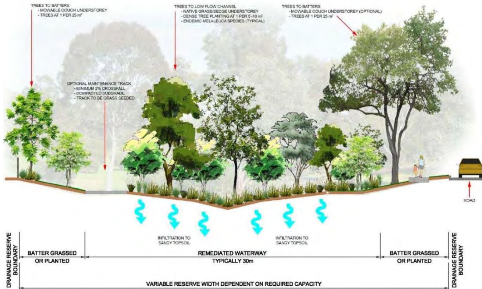
Figure 13: Remediated waterway typical section
