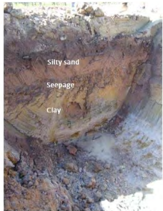
Photo: Shallow silty sand over sandy clay and clay
