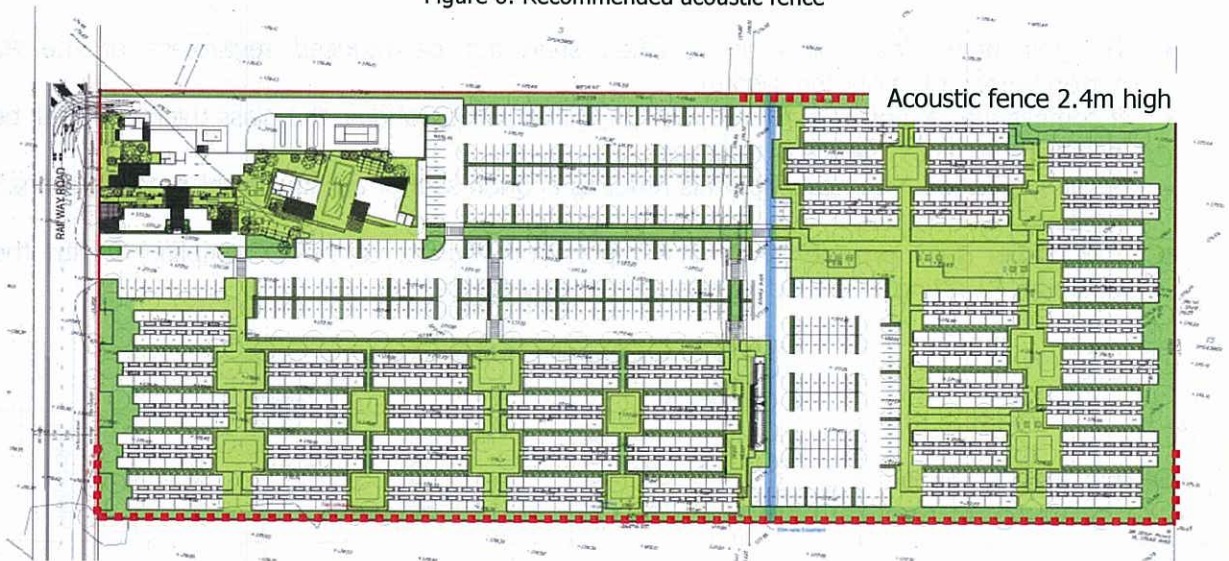
Figure 6: Recommended acoustic fence
