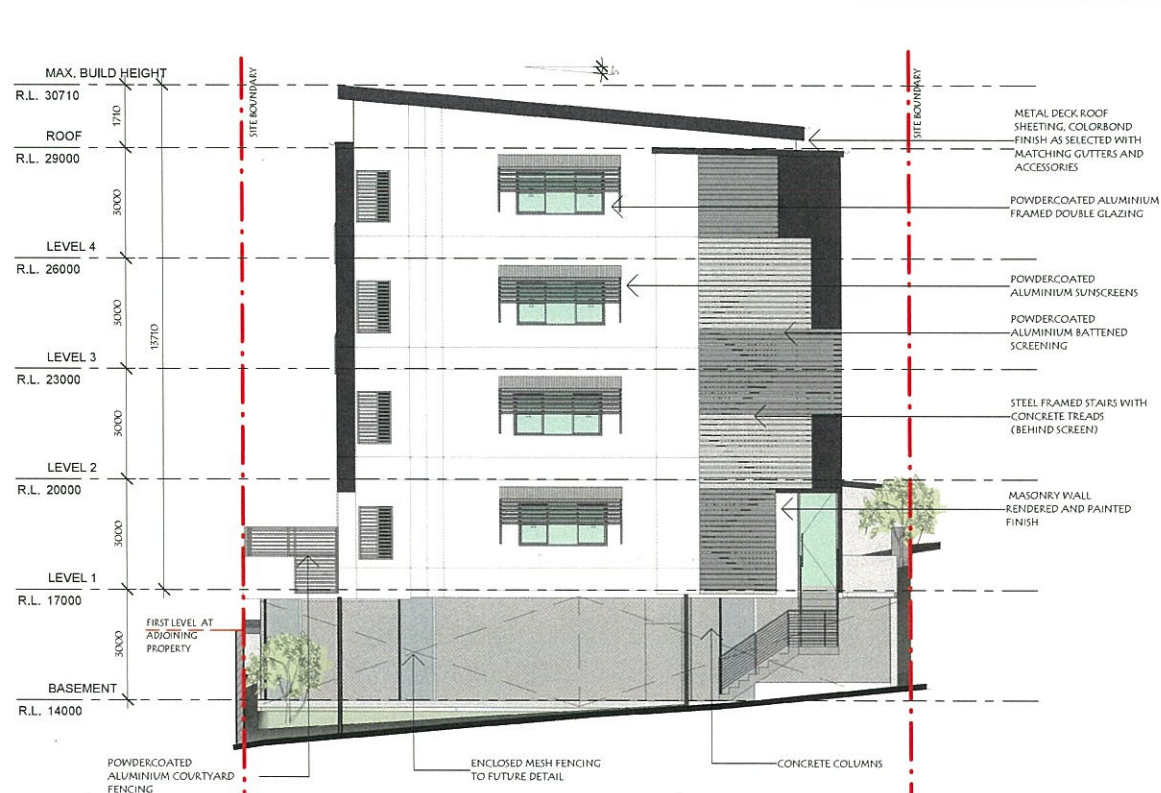
WEST ELEVATION MULTI-UNIT DEVELOPMENT 1:100
