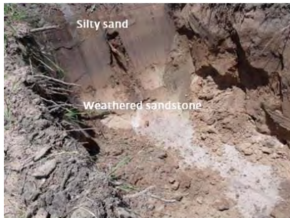
Photo: Silty sand over weathered sandstone
