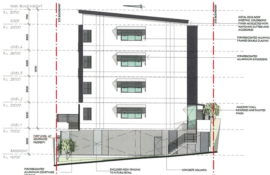
WEST ELEVATION MULTI-UNIT DEVELOPMENT 1:100
