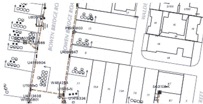
Figure A.2 - Existing Energex Electrical Records
