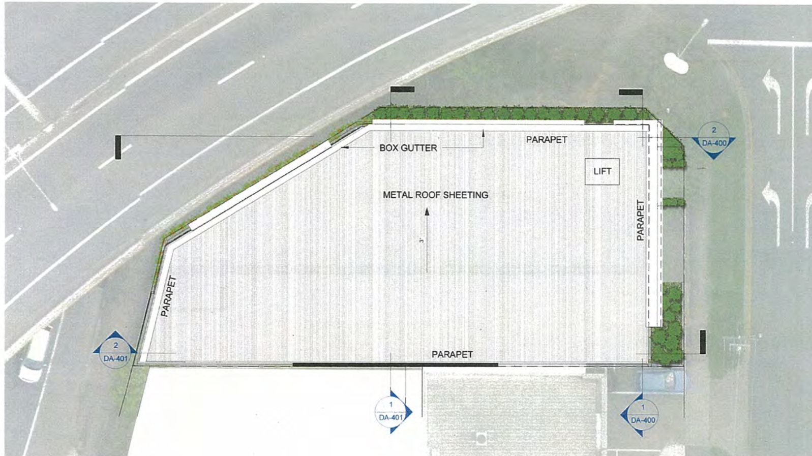
1 ROOF PLAN 1:200@A3
