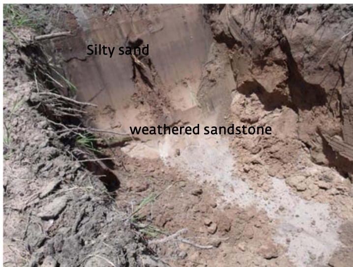
Photo: Silty sand over weathered sandstone
