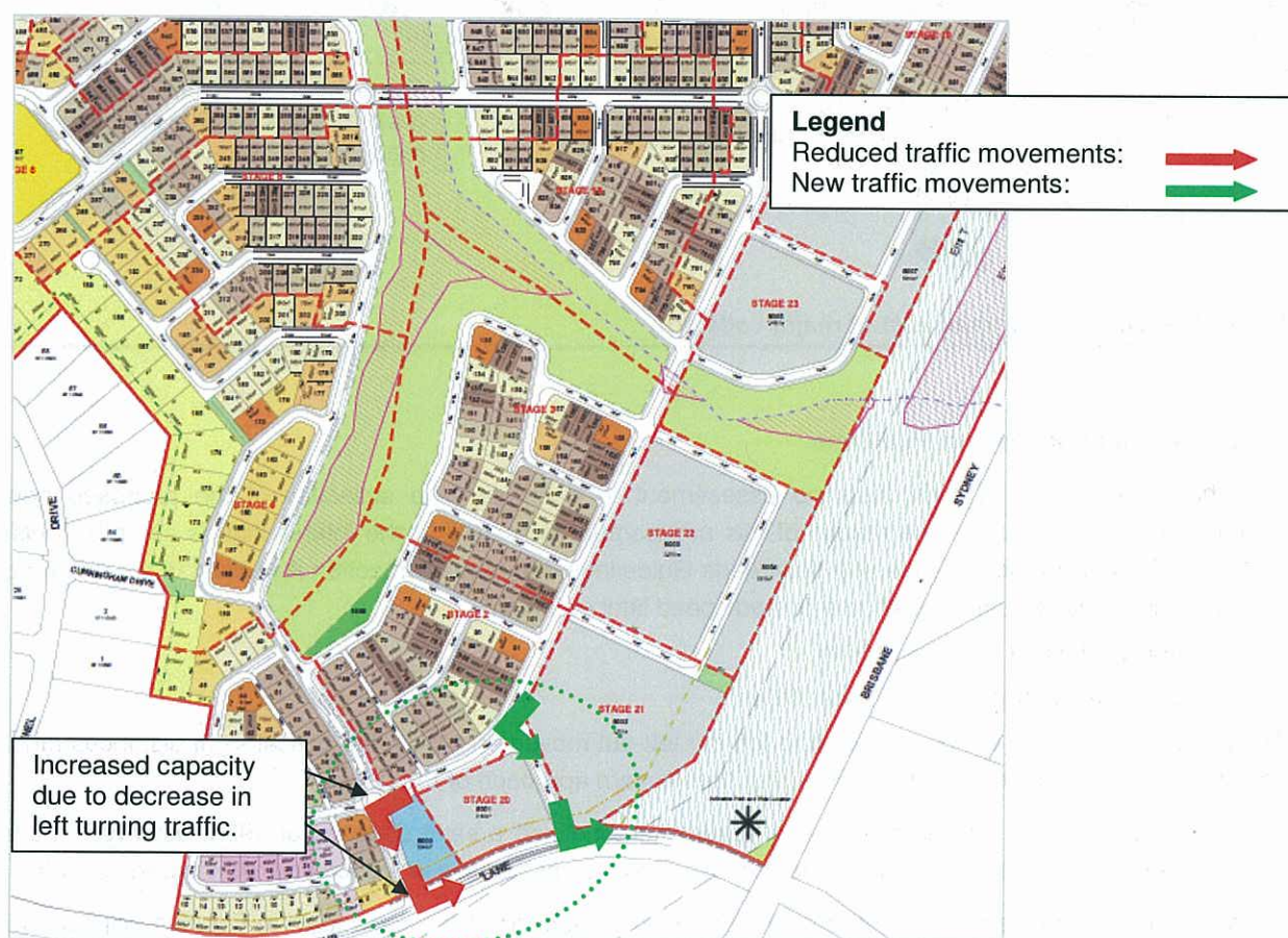
Figure 2: Localised changes in traffic movements
