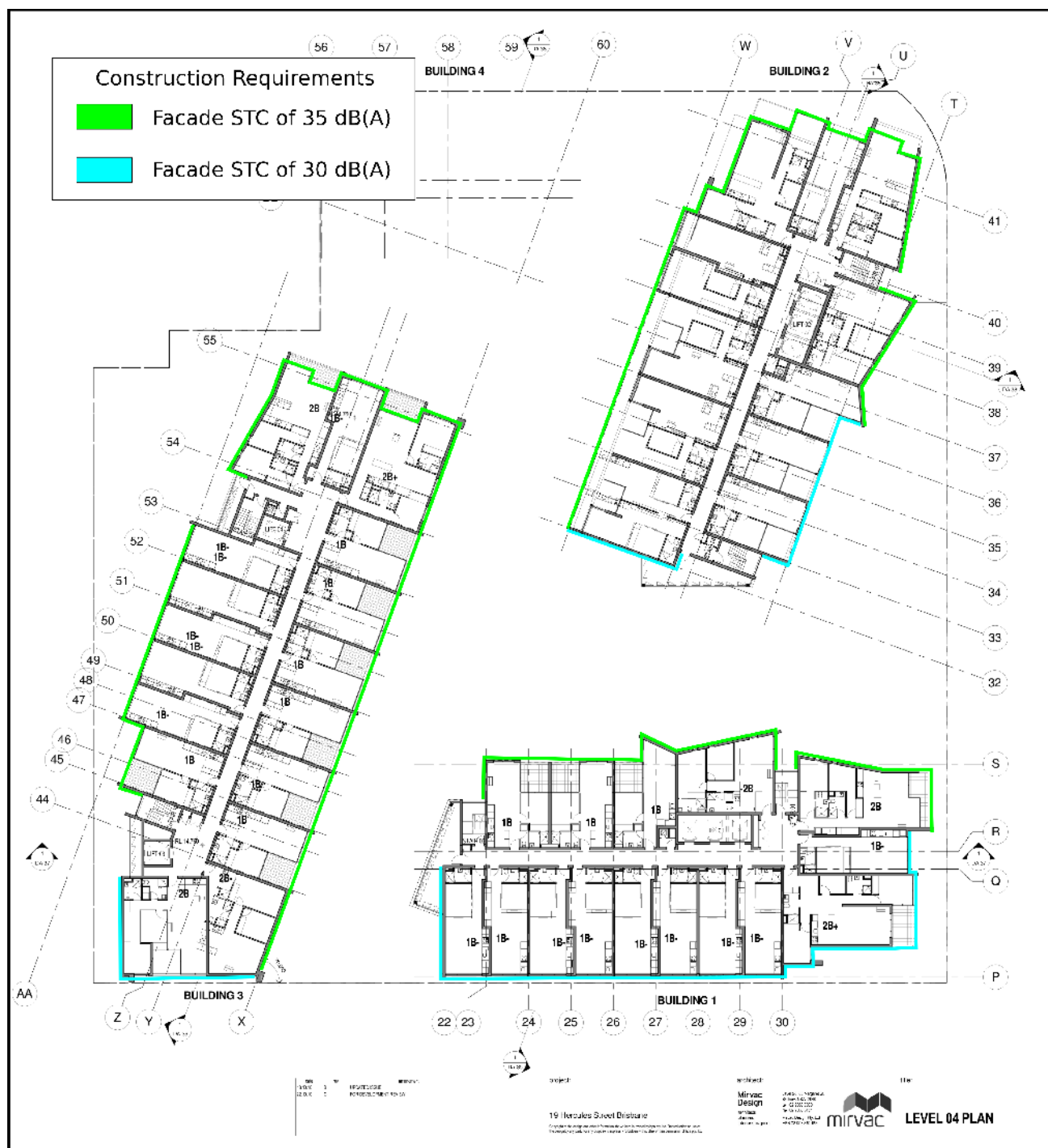
Figure 6: Facade Treatment Recommendations
