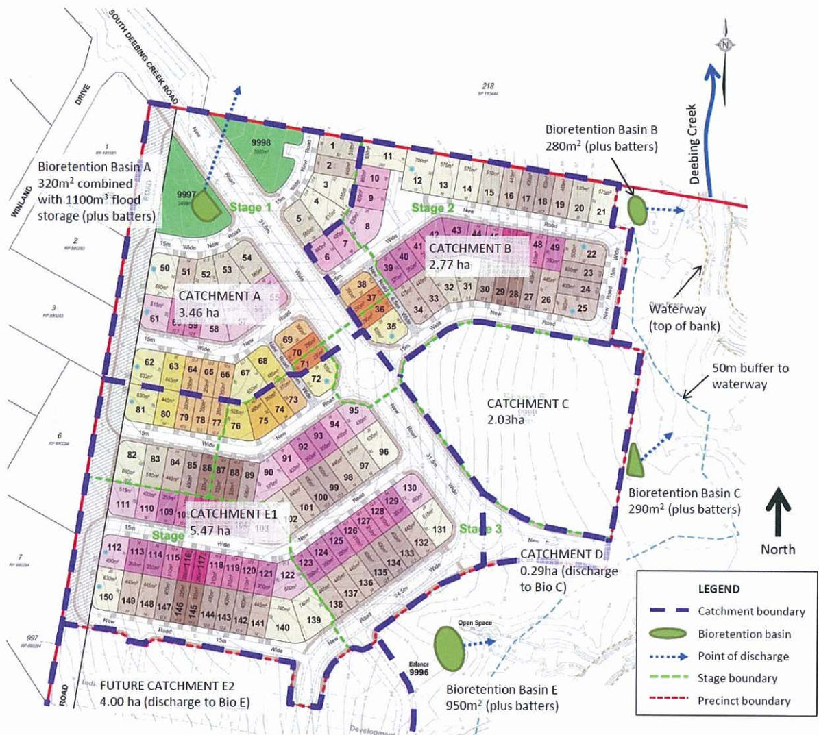
Figure 2: Original development plan and stormwater strategy
