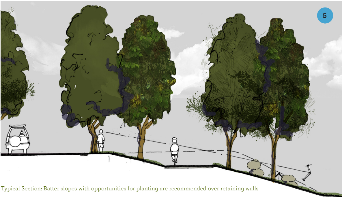
Typical Section: Activity Trail or Pedestrian Pavement adjacent to open space when upstand kerb is used
