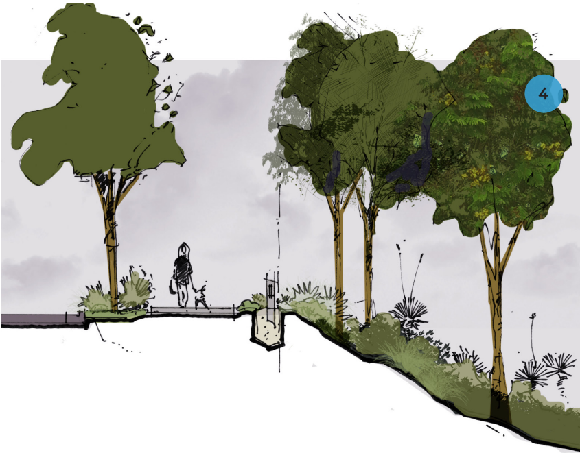
Typical Section: Activity Trail or Pedestrian Pavement adjacent to open space when upstand kerb is used
