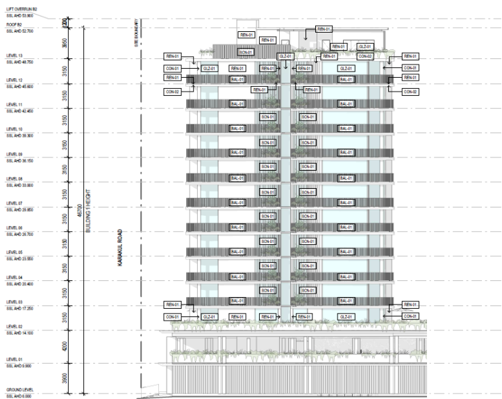
1 BUILDING ELEVATION - BUILDING 2 - WEST SCALE 1:250 @ A3
