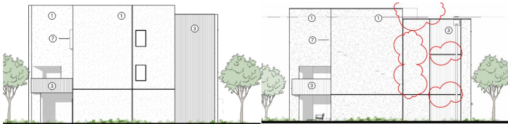
Figure 6: Building 2 LH End Condition, Before - Left, After - Right
