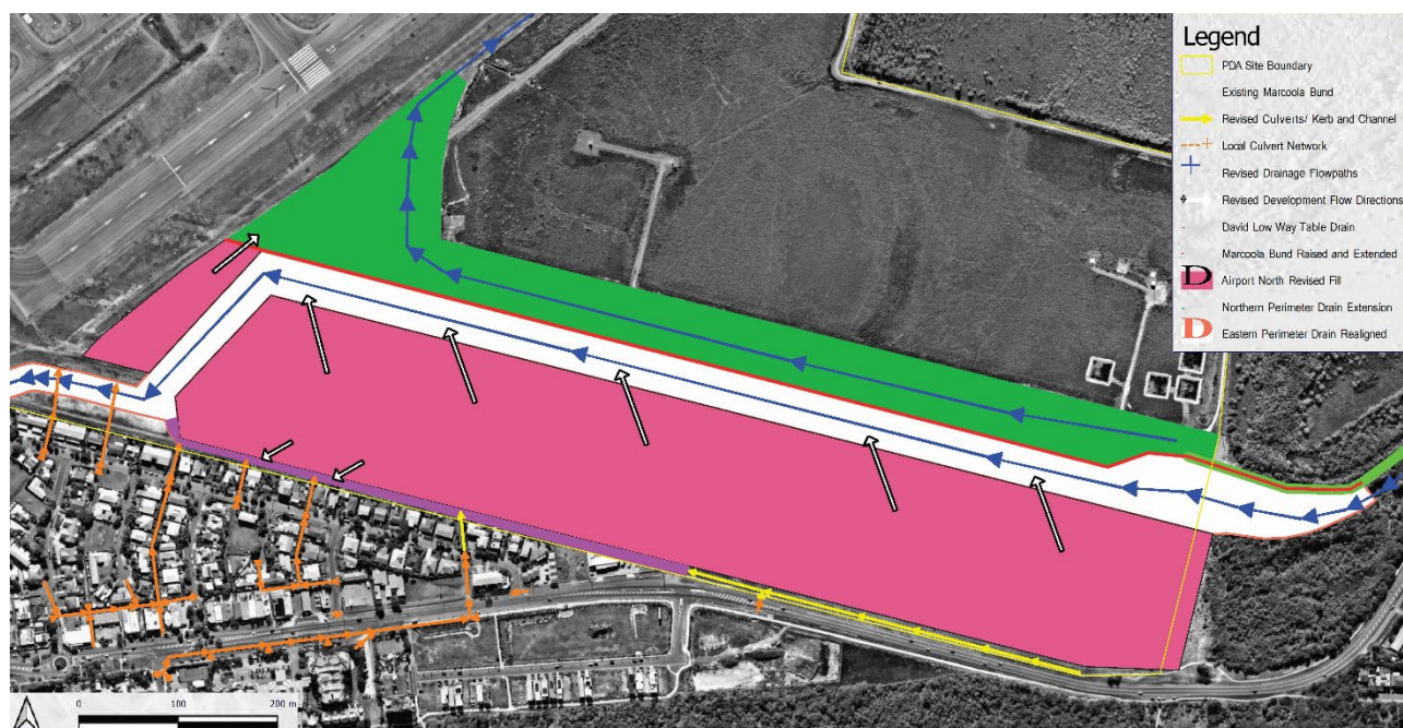
Figure 6: Proposed Airport North, East Perimeter Drain realignment
