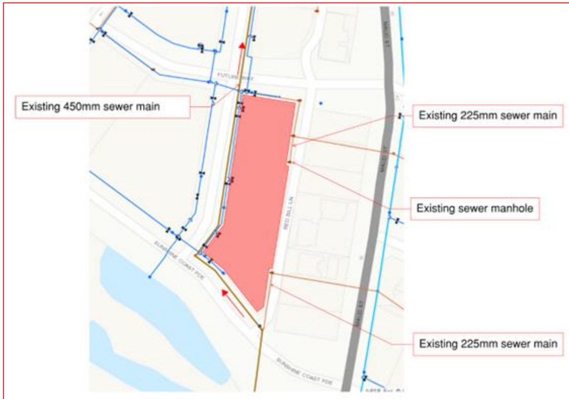
Figure 5: Existing sewer infrastructure
