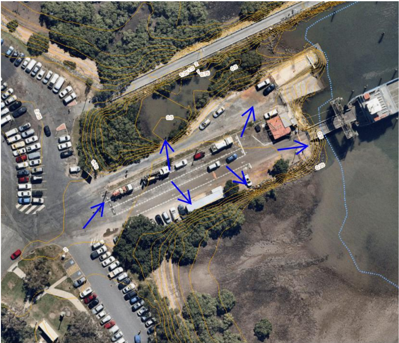
Figure 2-2: Site Topography and Drainage Features
