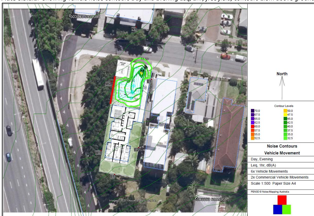
Plate 6.5.1.1: Showing vehicle noise contours Day and Evening Leq, 1hr, free field, contours 1.5m above ground.
