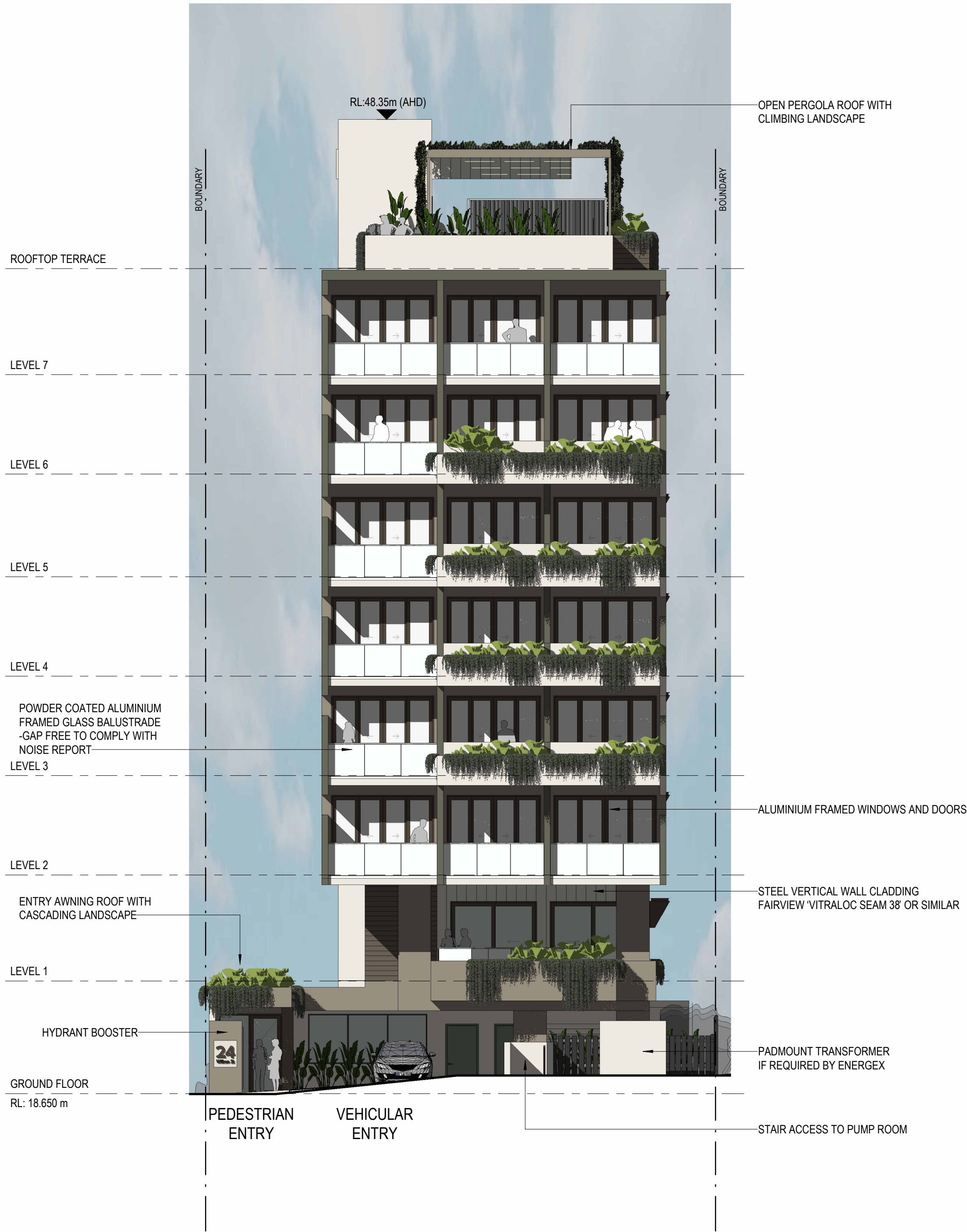
1 NORTH ELEVATION (WILTON STREET) SCALE 1 : 100 @ A1
