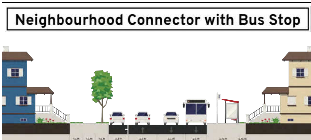
Figure 3.4: Neighbourhood Connector with Public Bus Stop Cross-Section
