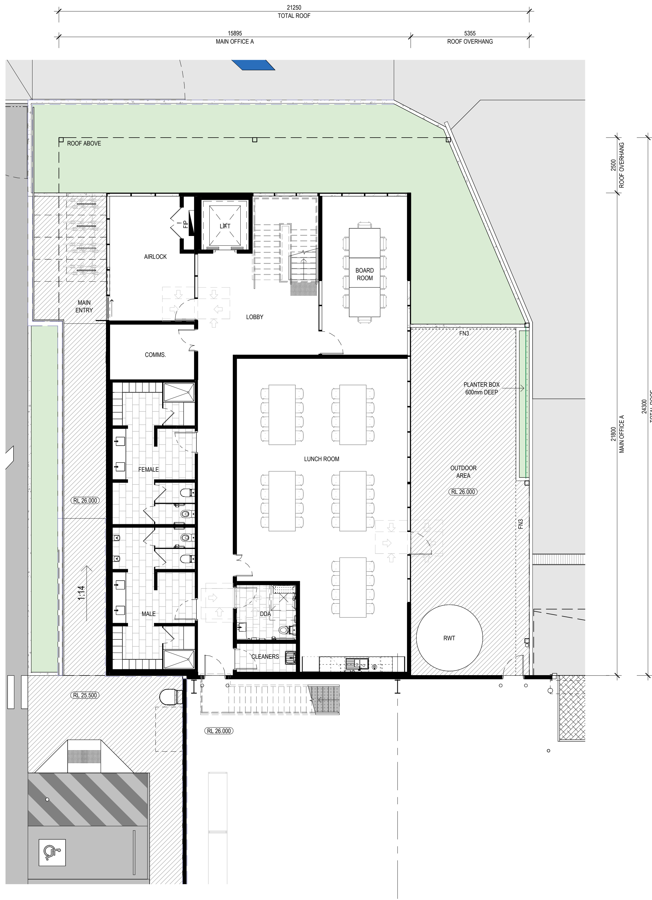
MAIN OFFICE GROUND FLOOR SCALE: 1 : 100
