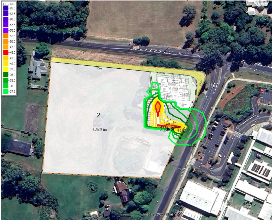
Plate B1: Noise contours at 1.8m, vehicle movements. Levels are in dB(A) Leq
