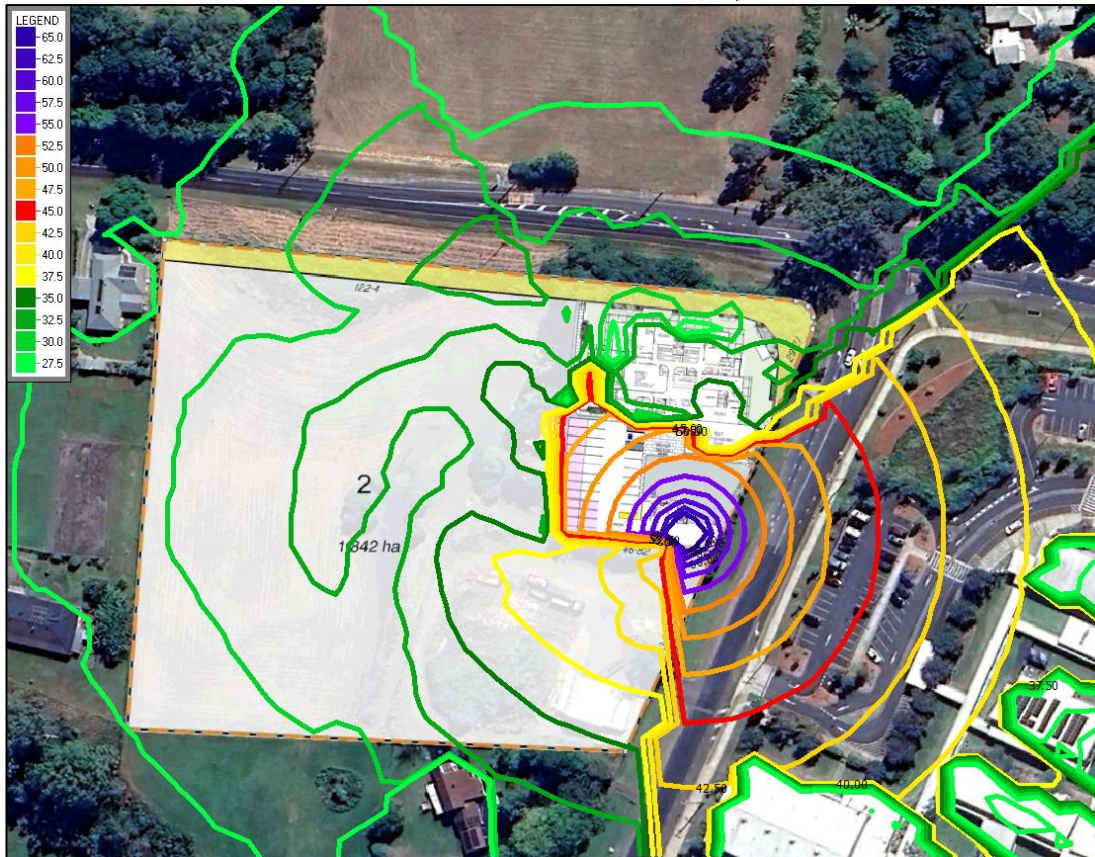
Plate B4: Noise contours at 1.8m, rubbish collection. Levels are in dB(A) L_{eq,15mins}
