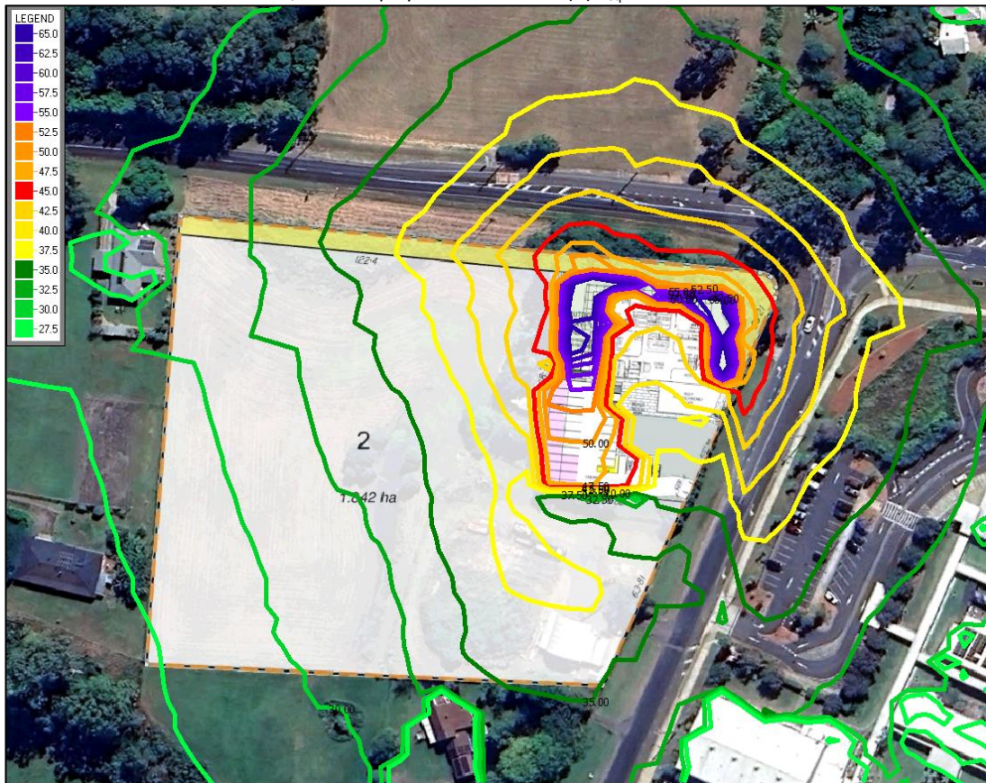
Plate B2: Noise contours at 1.8m, outdoor play. Levels are in dB(A) L_{eq}
