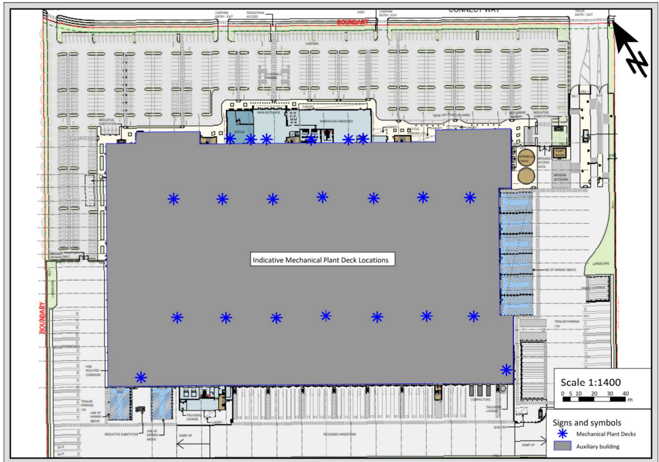
Figure 7-1 - Mechanical Plant Source Locations
