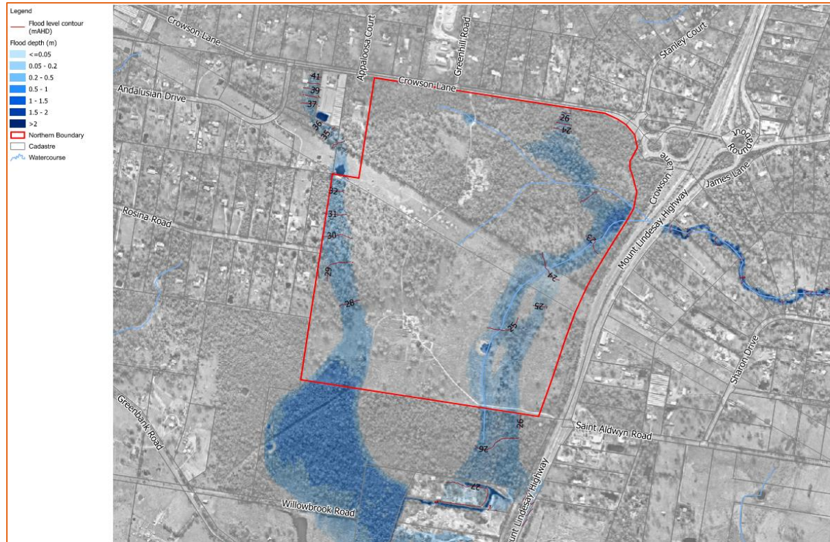
Figure 6-1 - Existing Peak Water Depth - 1% AEP
