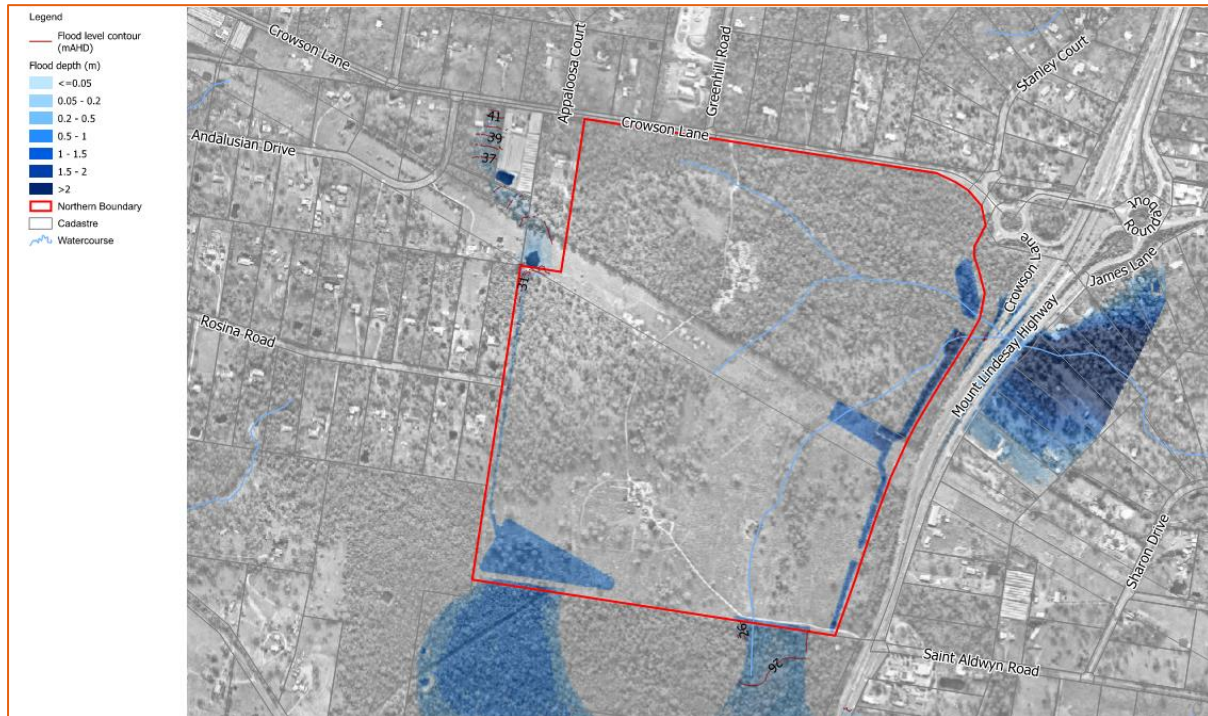
Figure 6-10 - 1% AEP 72hr Regional Flood Depth and Extents
