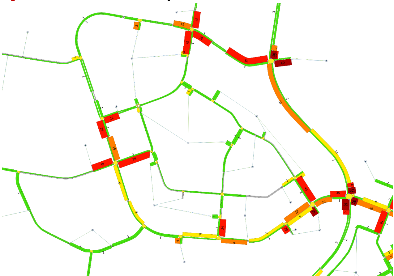
Figure 4.7: Microsimulation Link Delays - PM Peak
