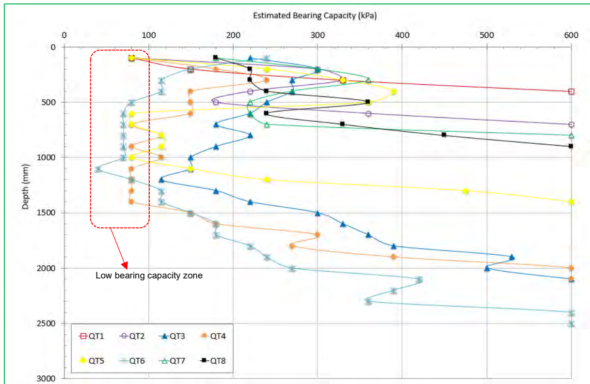
Figure 7: The Allowable Bearing Capacity of Onsite Soils with Depth; Derived from DCP Data
