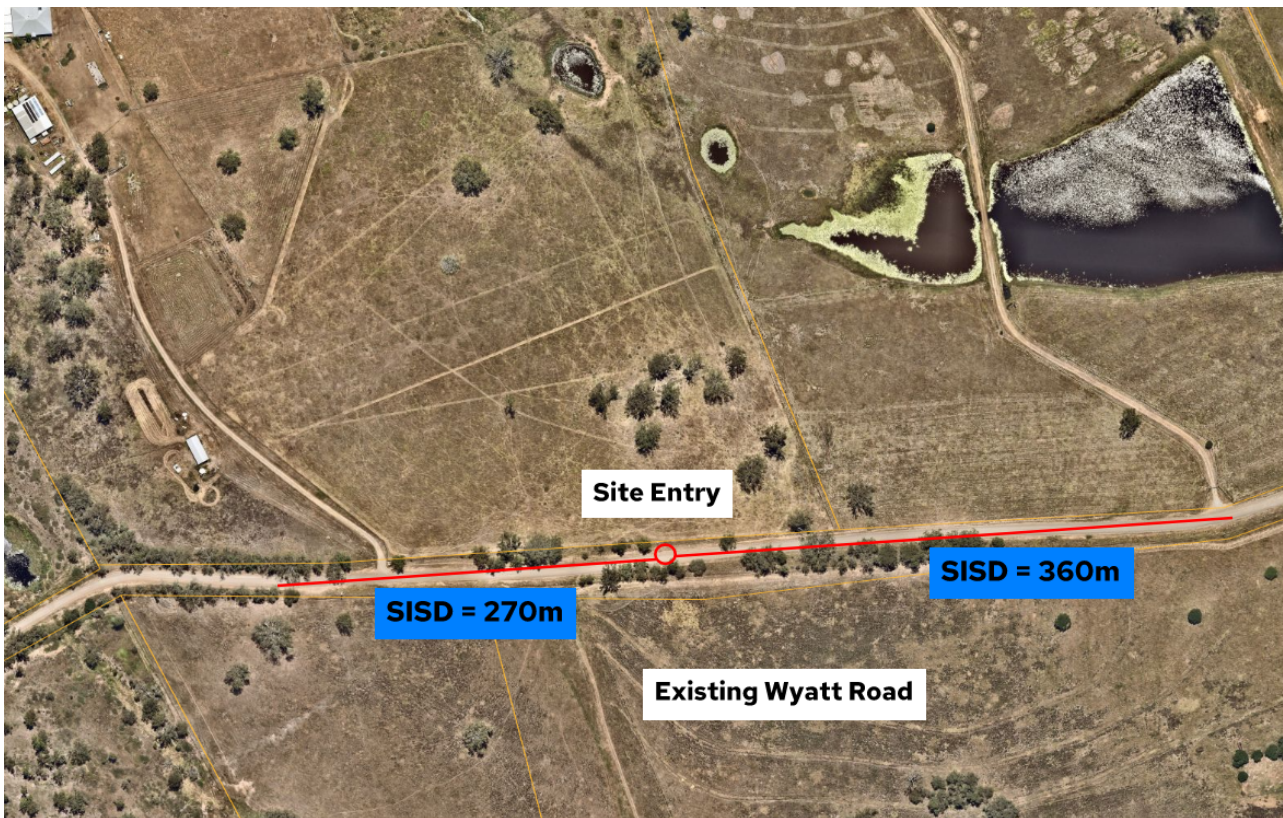
Figure 6.2 Sight line to Proposed Site Entry off Existing Wyatt Road
