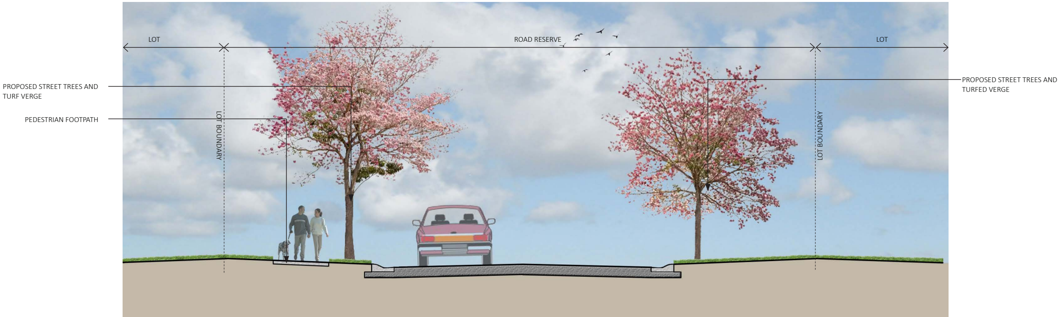
SECTION C 16m ROAD RESERVE PATHWAY SCALE 1:100 @A3
