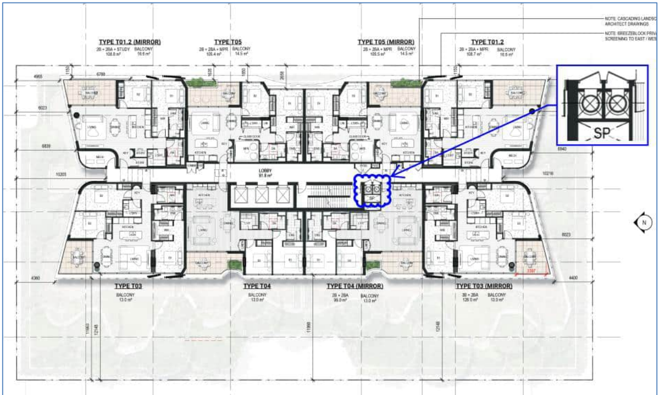
Figure 3-3: Typical Residential Level Chute Access to AWCS
