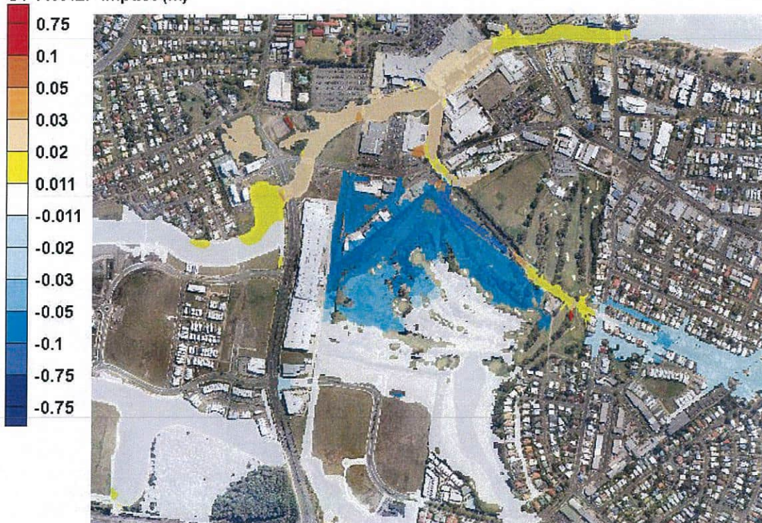
Figure 6 Stage 1 Temporary Works 1% AEP Flood Impact
