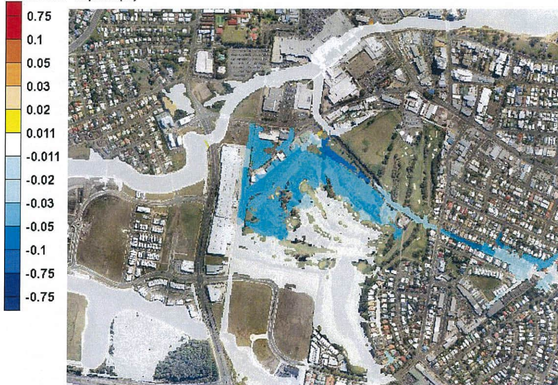
Figure 5 Stage 1 Temporary Works 2% AEP Flood Impact
