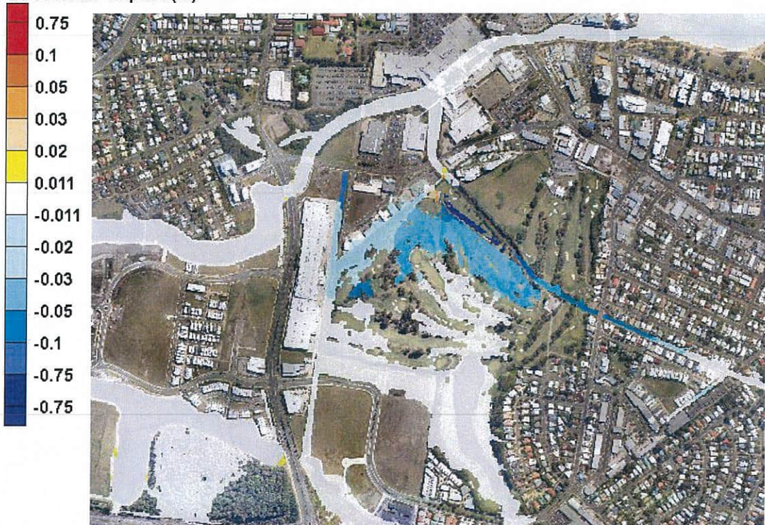
Figure 2 Stage 1 Temporary Works 18% AEP Flood Impact
