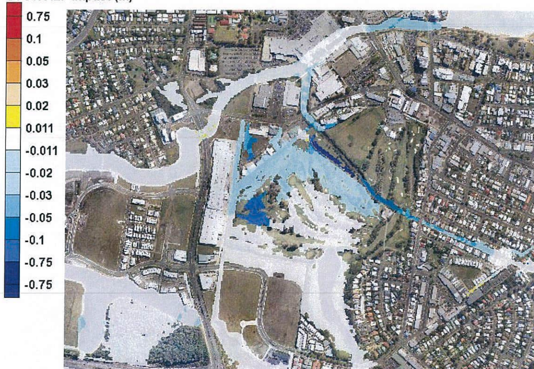
Figure 4 Stage 1 Temporary Works 5% AEP Flood Impact
