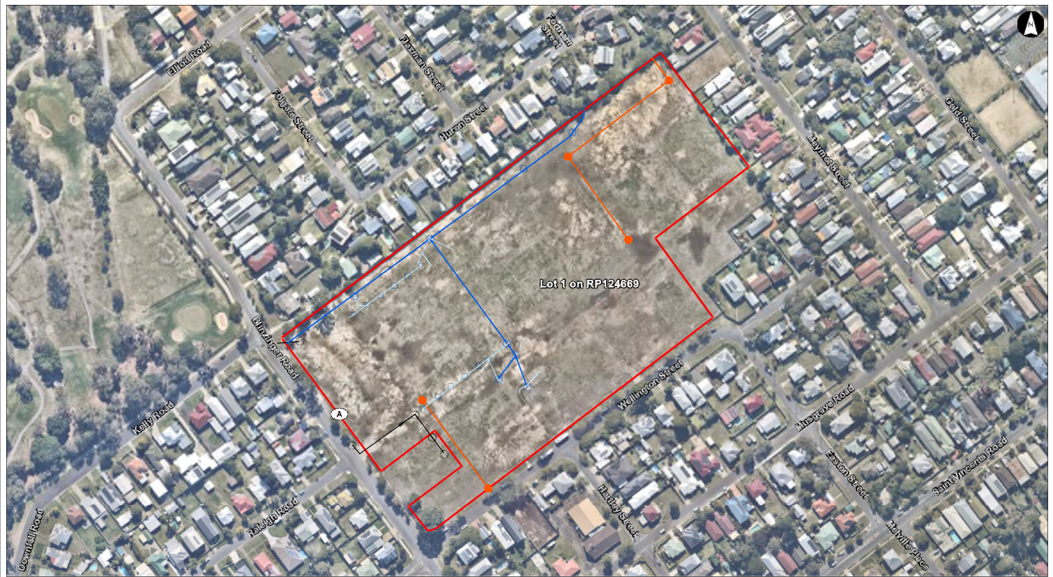
Figure 3 – Underground Services 56 BLININGER ROAD, BANYO
