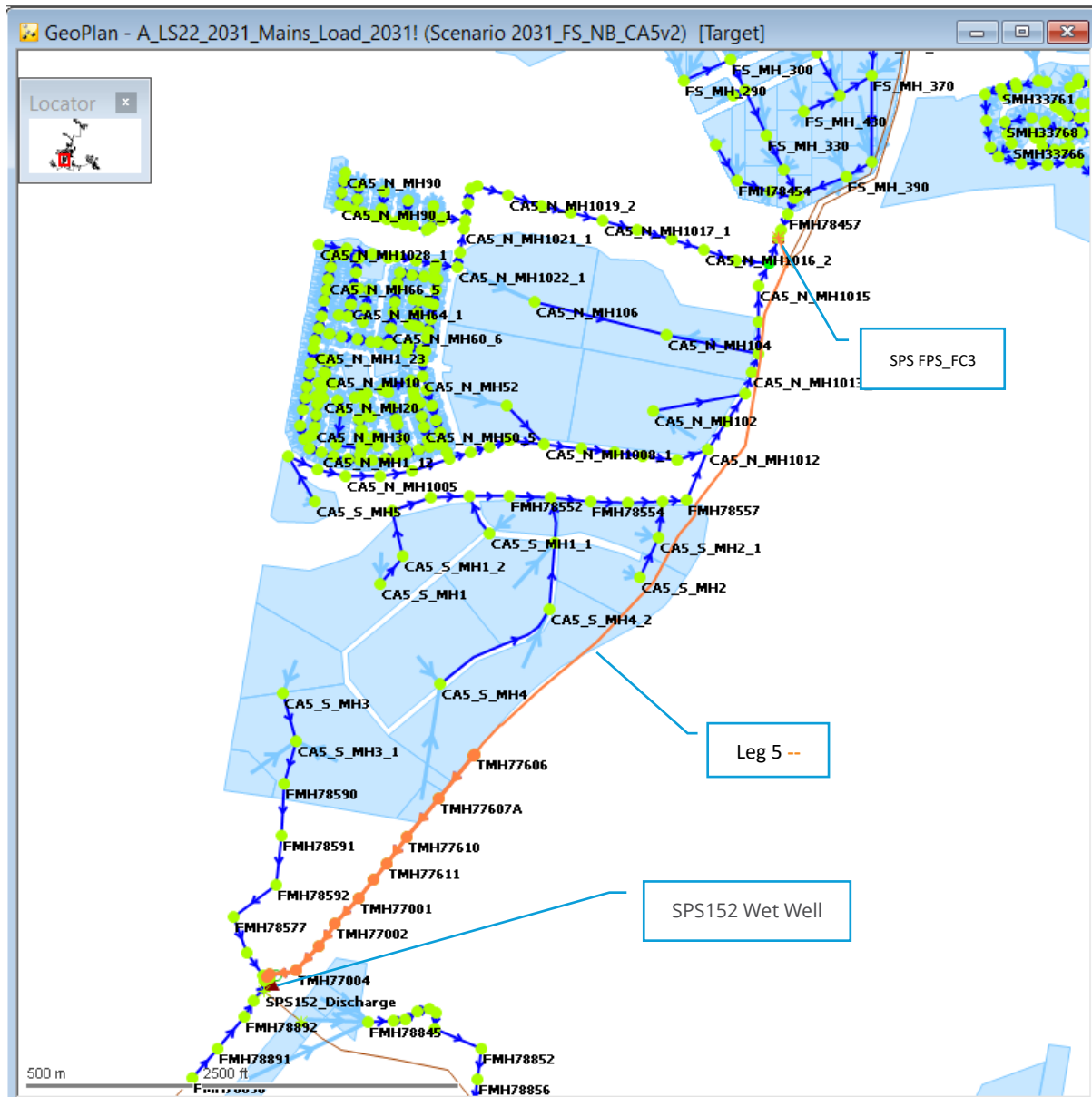
Figure 6-6: Leg 5 Sewer Network (2031 Planning year)
