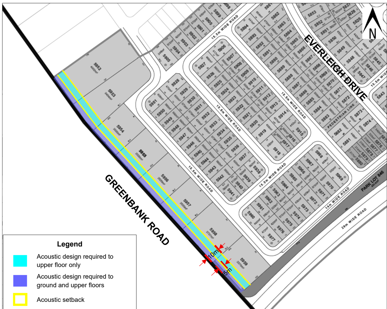
Figure 6.1 Noise control measures – RoL 7
