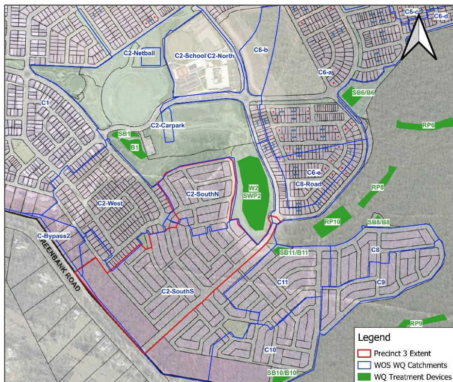
Figure 3: Precinct 3 Stormwater Quality Catchments
