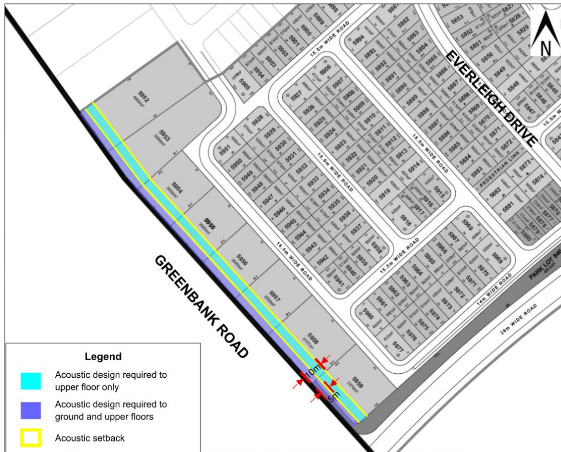
Figure 6.1 Noise control measures – RoL 7
