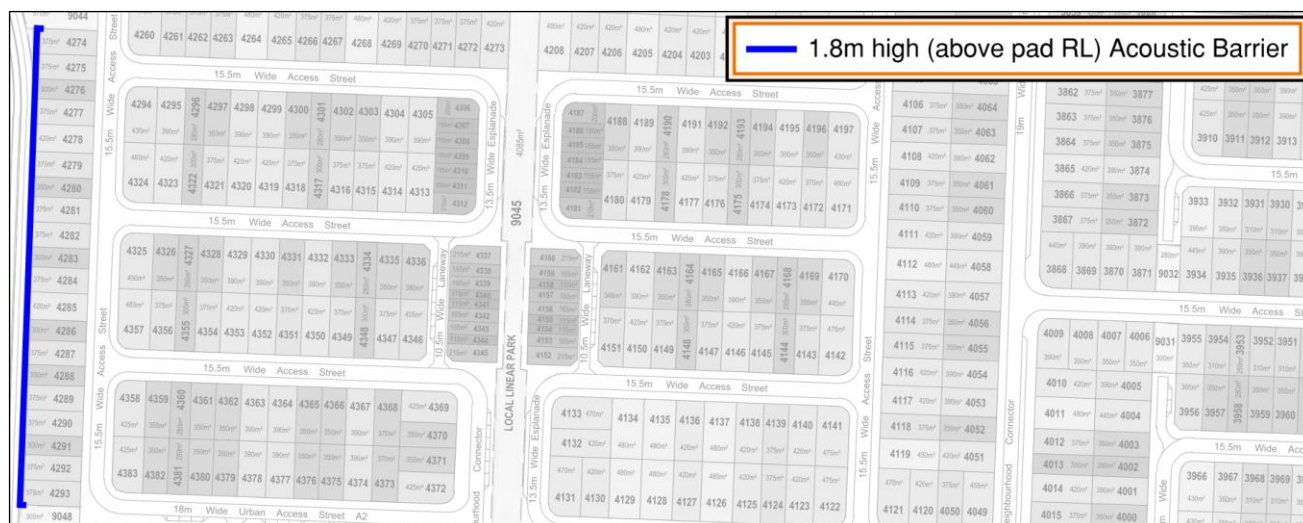
Figure 12: Proposed internal road acoustic barriers (Northeast Section)
