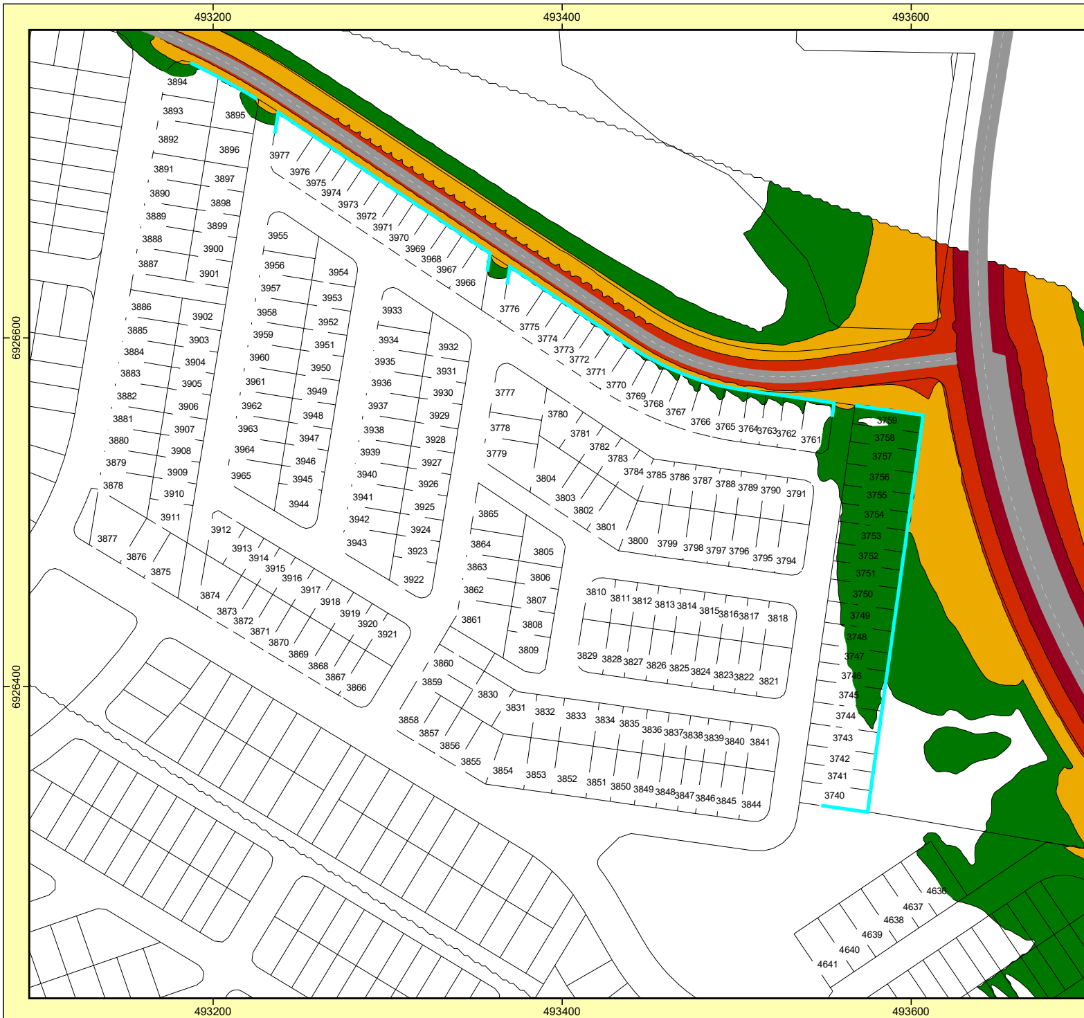
Figure 7 - QDC MP4.4 Noise Categories 2041 Road Traffic Noise Levels Ground floor noise prediction at 1.8m above the ground with 2.0m high noise barriers
